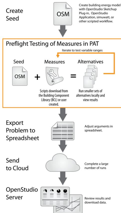
Figure 1 OpenStudio Parametric Workflow
